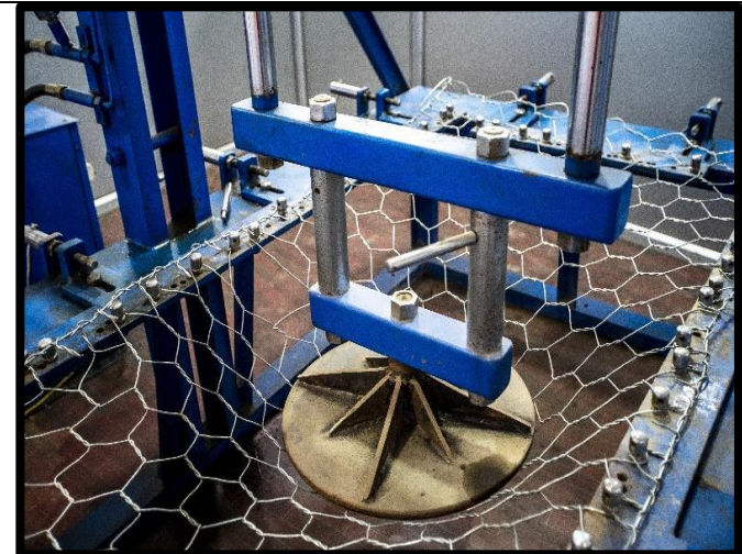
Punch Strength testing of Rockfall Netting. This determines the effectiveness of netting to protect against dislodging rock.
